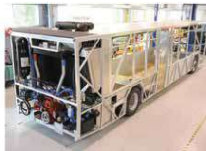
Photograph of the Optimized Bus Frame
